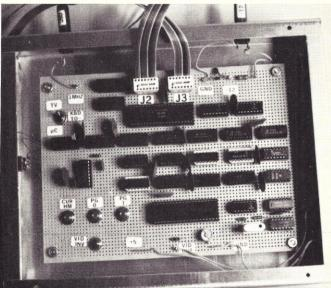
Finished terminal on a  $6 \times 8$  inch perfboard mounted in an  $8 \times 10$ inch chassis box. Note that there was enough room to mount most of the switches on the perfboard. J2 goes to my keyboard, while J3 goes to the SYM-1. Next to "VID OUT" is C3, which adjusts the line width. I recommend using labels for all devices and terminals.
